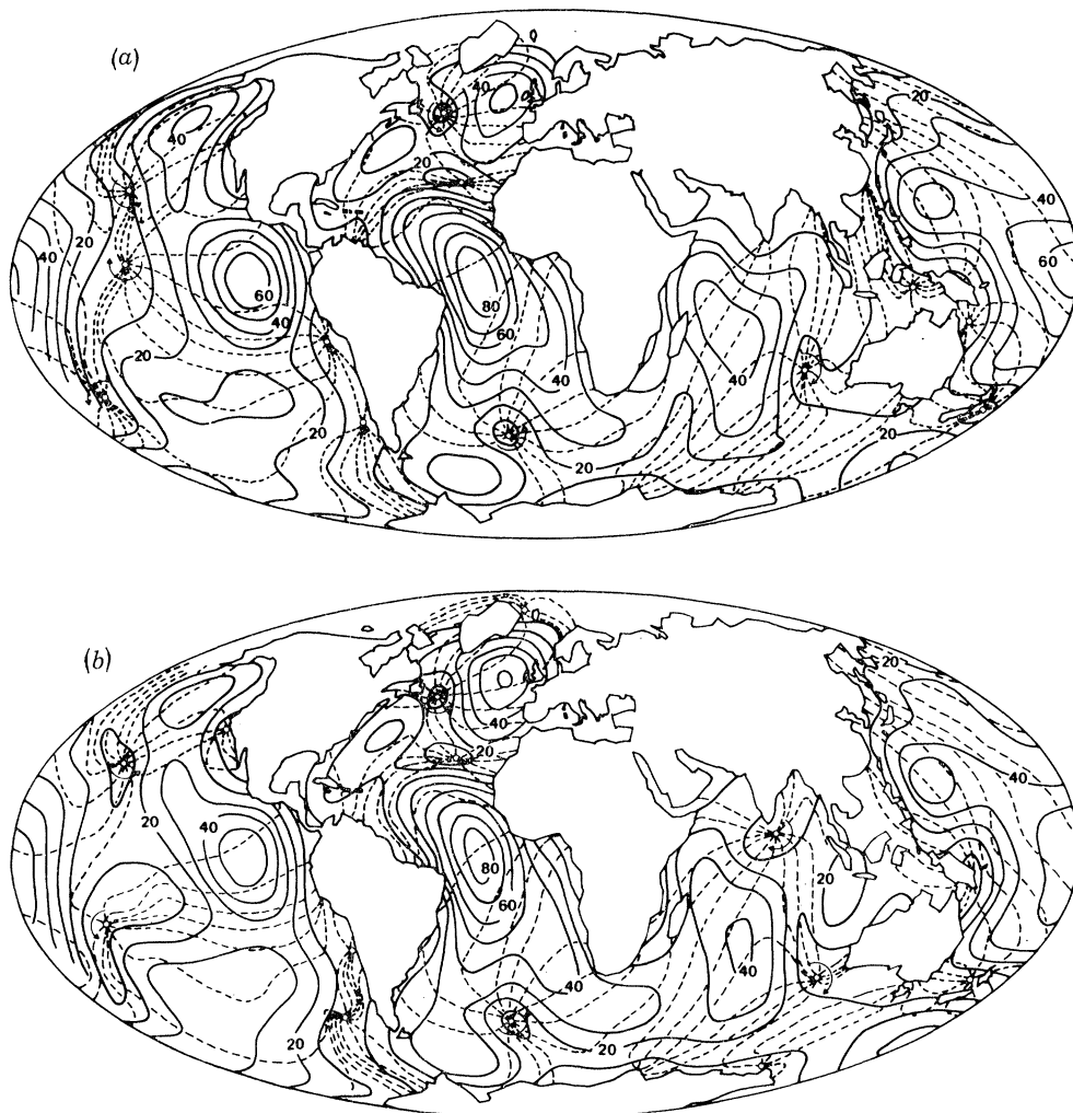
FIGURE 3. (a) Numerical model of Bogdanov & Magarika expressed in spherical harmonics up to degree and order 10. (b) The combined Bogdanov–Magarika and satellite solution expressed in spherical harmonics up to degree and order 10.
